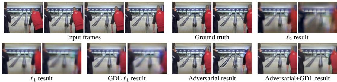
Figure 3.7: Comparison of different loss function combinations using a simple CNN to predict one frame given four inputs. The second future frame is predicted recursively. (From [MCL16])
